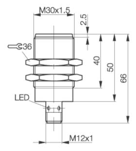
**Inductive Sensors BES M30EG1-PSC80S-S04G-S** M30x1.5 x 66 normally-open Sn=8mm shielded
